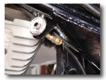
3. Use the  $\frac{1}{4}$ " air line supplied in the kit and simply push it into the "push to connect" fitting that's already installed as part of the pressure gauge assembly.
