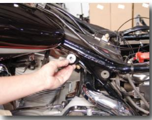
2. Use the existing 1/4" hole in the underside of the frame, in front of the battery box, to mount the pressure gauge.
