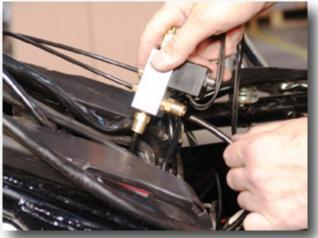
4. Route the ¼" line from the gauge, rearward through the large hole in the frame and connect to the distribution manifold. You will need to remove the plug and insert the fitting supplied in the kit. Cut the ¼" air line to length and connect.
