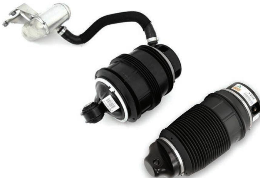
**The A-2725 Eliminates The Need For An Air Reservoir.**
